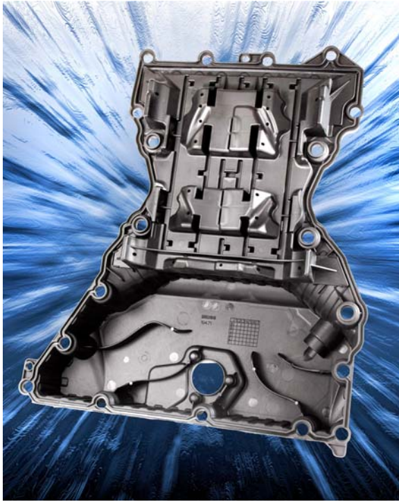
Figure 12. For the first time in automotive history, an oil pan module made from a thermoplastic polymer is now used for commercial production vehicles. The combination of modulus as a function of temperature, impact resistance, and relative compatibility with hot engine oil contributed to the selection of Zytel® 70G35HSLR for the oil pan module of the 4-cylinder diesel engines of Mercedes-Benz C Class vehicles.
