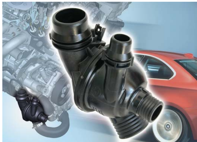
Figure 3. The housing of the map-controlled thermostat by Behr Thermot-tronik, which is installed in BMW's N43 series four-cylinder petrol motors, is exposed to very high mechanical, thermal, and chemical stresses. Automotive coolant flows through the interior of the thermostat housing at temperatures up to 140 °C. The combination of high temperature coolant resistance, creep performance, and resistance to typical motor-compartment media (such as oils, greases, fuel, and road salts) contributed to the selection of Zytel® HTN51G35HSLR for this engine-mounted component.
