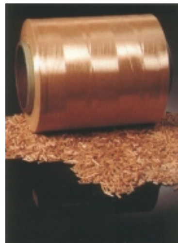
Fig. 1: Pellets, 1/2-in, long, are made from continuous aramid yarn meltcoated with nylon-66.
