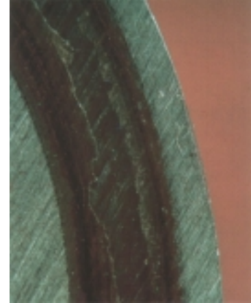
Glass-filled nylon has high/abrasive effect on this finished steel washer surface.
