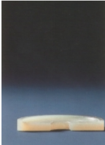
Unreinforced ZYTEL® resulted in a wear factor of 18.5 -wearing 4X faster than parts reinforced with KEVLAR® RTP.
