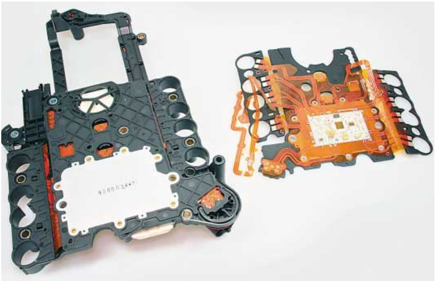
Left: The platform of Zytel® seen from the underside. Right: the flexible circuit, based on a Pyralux® carrier laminate.
