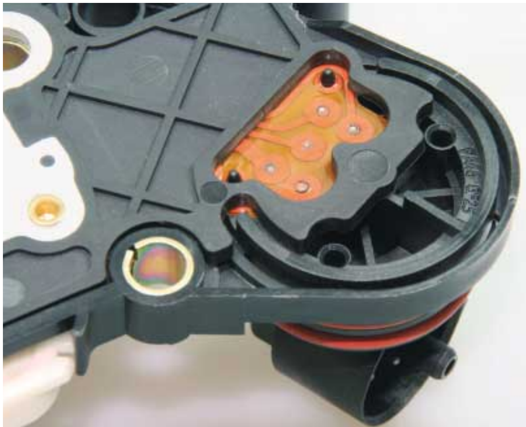
At the board's outer edges the Pyralux® laminate is connected to sensors or actuators
