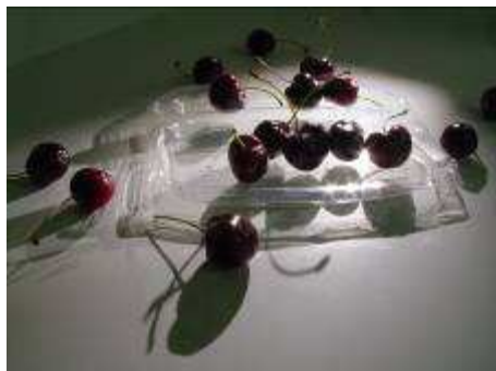
Formed PLA Tray without additive – heated to and kept at 70°C for 1 hour
