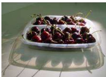
Formed PLA Tray with 2% Biomax® Thermal 300 – heated to and kept at 70°C for 1 hour
