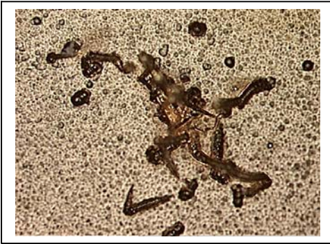
Figures 5 & 6: Optical Microscope Pictures of "Stringy Nodules"
