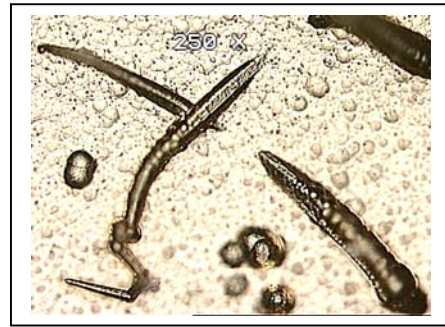
Figures 5 & 6: Optical Microscope Pictures of "Stringy Nodules"
