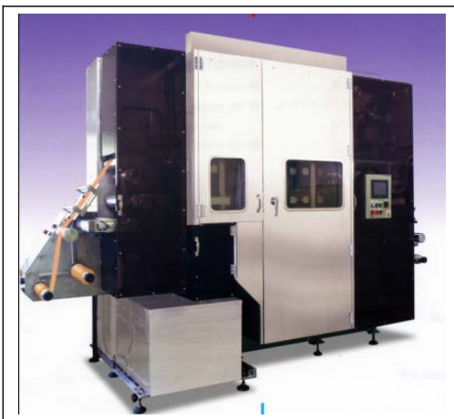
Fig. 4: Dip coater for flex circuits (FPC) FD-0411 (Source: SDI Company Ltd)
