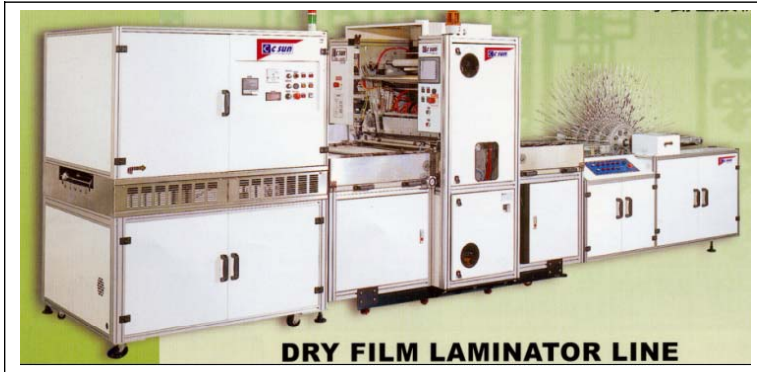
Fig. 3: Dry Film Lamination Line (source: C Sun)
