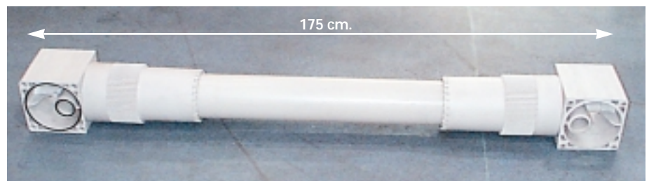
USF Memcor® Continuous Microfiltration system (CMF) filter housing uses a centre tube and head pieces of injection moulded from a toughened PA612 grade of Zytel® with 33 per cent glass reinforcement. End caps, spacers and outer sleeves are moulded from a second toughened PA612 grade of Zytel®, also with 33 per cent glass reinforcement.
