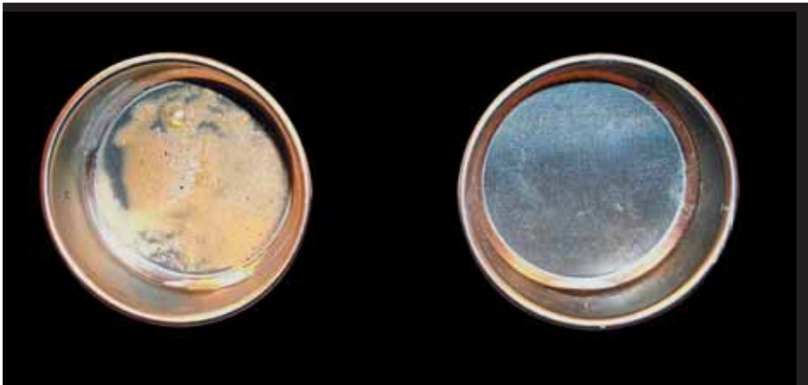
Figure 2: 75 micron (200 mesh) wet sieve retains. The diameter of the sieve is 10 cm (4 in). Generic chlorsulfuron (left). DuPont™ Telar® DF herbicide [chlorsulfuron] (right).
