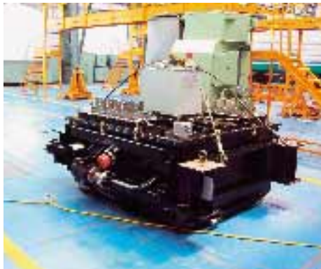
Oil filled traction transformer. Power: 6 MVA. Weight: 6 tonnes.
