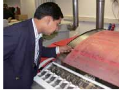
Mr Chaudhary looking the plate's quality coming out of the Cyrel® FAST 4260 thermal processor.
