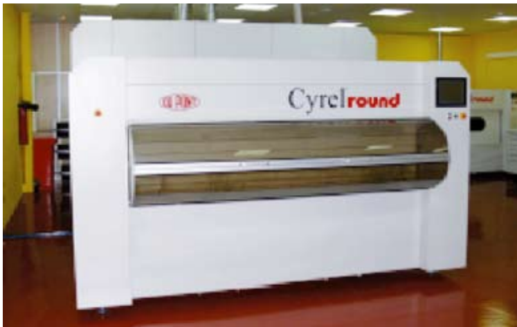
The latest Diflex investment: a Cyrel® round solution to produce seamless sleeves for high precision and quality packaging printing.
