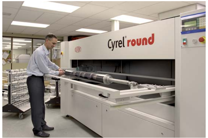
"Dave Kershaw, Business development manager PPP, maintains a keen interest in production and can be seen inspecting a Cyrel® round sleeve prior to UV exposure."
