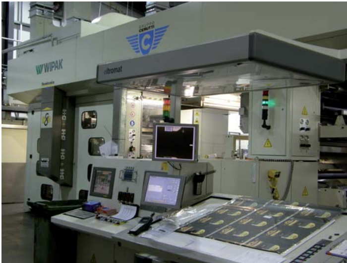
"Wipak's latest press, the Flexotecnica, uses Cyrel® round and the Eltromat automatic register system to deliver outstanding register - fast."
