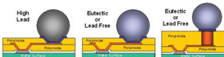
Figure 1 WL-CSP Dielectric Layer
