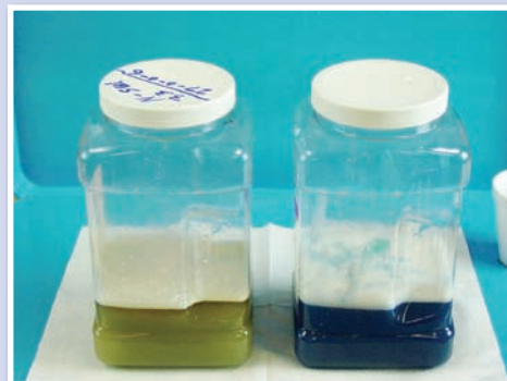
The jar on the left is incompatible. The jar on the right is compatible.
