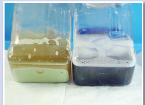
Note the precipitate in the jar on the left. These jars are different lots of the same 27-0-0-6 fertilizer.
