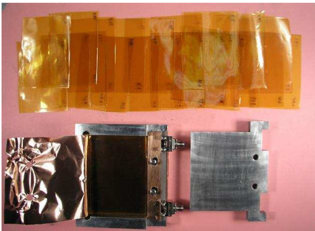
Figure 4 – Close-up of fixture showing individual layers prior to stacking.
