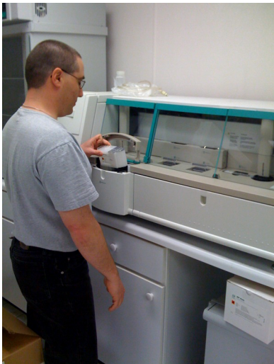
Michael DeCesare loads disposables into the automated RiboPrinter® System at Daniele Inc. food quality laboratory.
