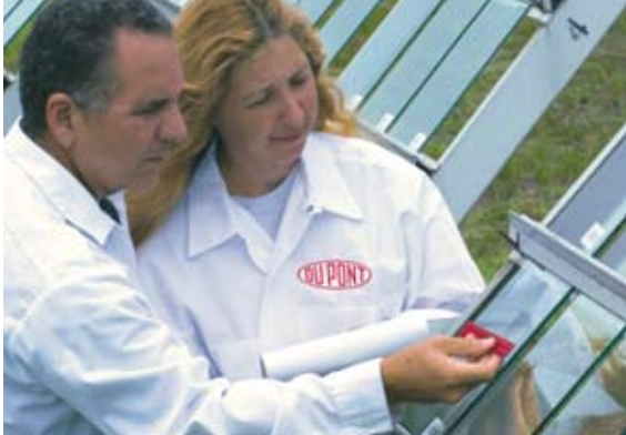
Edges of laminated glass test samples after weather exposure show no measurable moisture intrusion or delamination effects in open-edge application.
