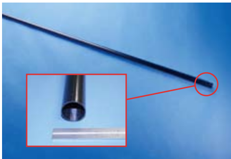
Hollow 3-D end effector design
