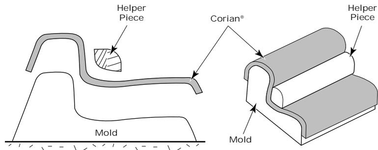
5. An option is to use a male mold in combination with a female mold.
