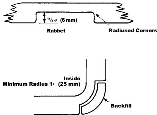
This reduces the thickness of the sheet in the inside radius section from  $\frac{1}{2}$ " (12 mm) to  $\frac{1}{4}$ " (6 mm), and the radius can be reduced from 3" (76 mm) to 1" (25 mm).
