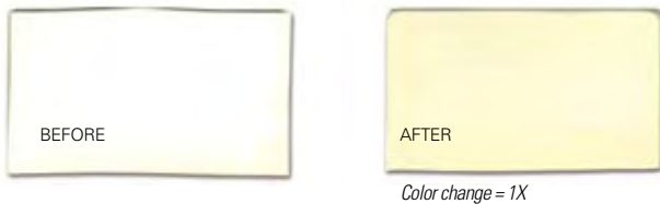
Figure 5: Discoloration of LDPE with Additives After UV Exposure
