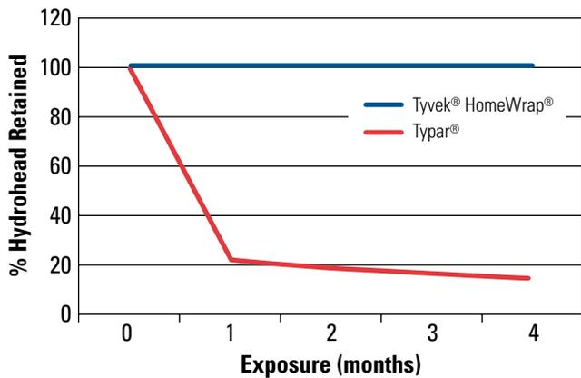
Figure 6 illustrates the effects of outdoor UV exposure on the performance of Typar® and Tyvek®. With as little as one month of exposure, Typar® lost most of its water resistance. After 4 months of exposure, Tyvek® maintained all of its water resistance.
