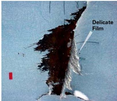
The film layer used with Typar® is weak and routinely damaged in the field. When damaged, the product offers little protection for a wall system.
