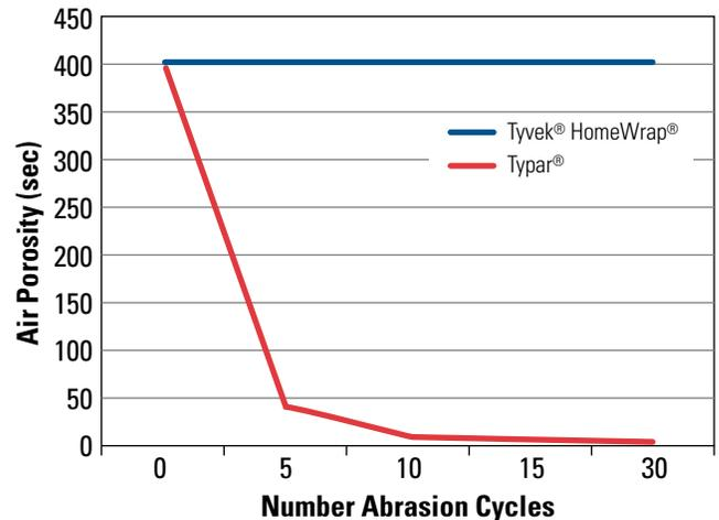
Figure 5 illustrates the effects of abrasion on the air resistance of Typar® and Tyvek®. After as little as 5 cycles, Typar® lost all of its effective air resistance. Tyvek® was not affected after 60 cycles.
