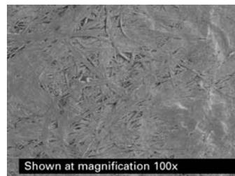
The Tyvek® structure on the left consists of very fine fibers which are fused together to produce an engineered sheet that does not require a coating or film for protection.
