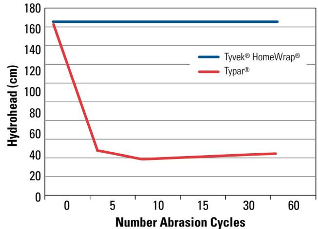
Figure 4 illustrates the effects of abrasion on the water resistance of Typar® and Tyvek®. After as little as 5 cycles, Typar® lost most of its effective water resistance. Tyvek® was not affected after 60 cycles. Test conducted per ASTM D3511.
