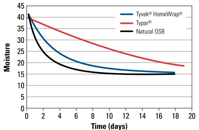
Figure 8 illustrates the ability of wall components to dry when covered with Tyvek® or Typar®. Tyvek® allows the OSB to dry significantly faster than Typar®.
