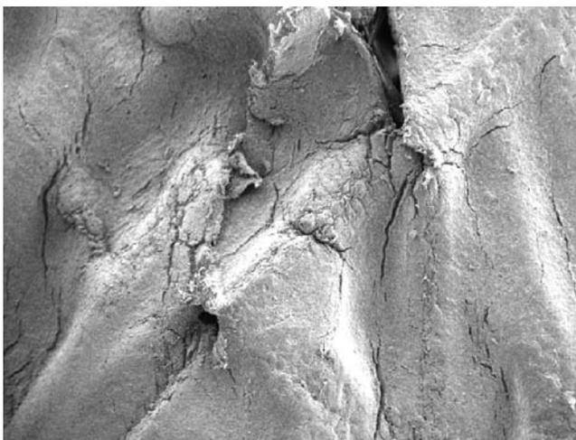
Figure 7 shows the effects of weathering on the Typar® film layer. Cracks and damage occur throughout the film layer, which allow water and air to penetrate.
