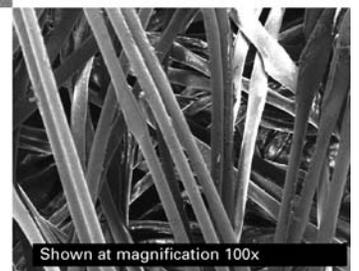
A multi-layer product like Typar® is only as good as its weakest component. The film layer is delicate and routinely compromised in the real world through tearing and abrasion (See Fig. 3). Unfortunately, this fragile film is what you would rely upon to protect the homes you build, and ultimately your reputation. The Tyvek® structure is unique and does not require a film or extra layers to perform, therefore there is no compromise.
